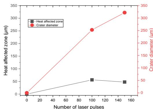
Fig. 4. Heat affected zone and crater diameter as a function of laser pulses.
