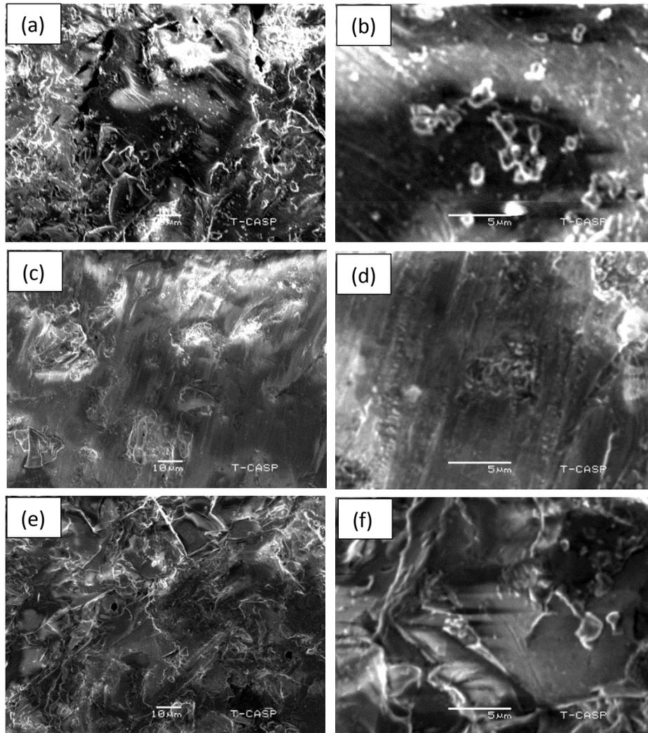
*Fig. 2. SEM micrographs of e.max Ceram samples (a) unirradiated (x1k), (b) unirradiated (x5k), (c) irradiated with 100 laser pulses (x1k), (d) irradiated with 100 laser pulses (x5k), (e) irradiated with 150 laser pulses (x1k) and (f) irradiated with 150 laser pulses (x5k).*
