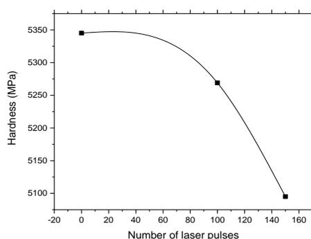
Fig. 5. Hardness of e.max Ceram as a function of the number of laser pulses.
