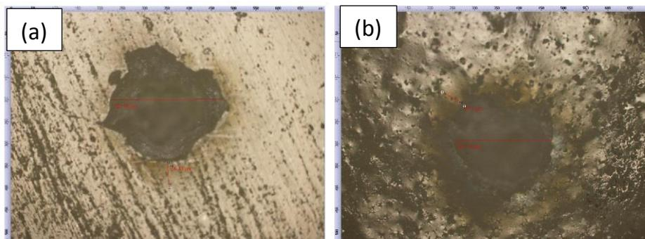
Fig. 3. Optical micrograph of e.max Ceram samples at  $\times 5$  (a) irradiated with 100 pulses and (b) irradiated with 150 pulses.
