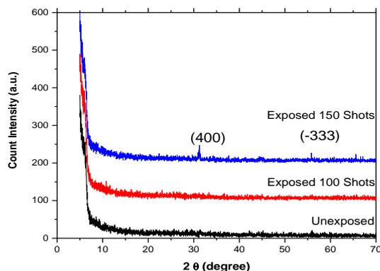
Fig. 1. XRD pattern of un-irradiated and irradiated e.max Ceram.
